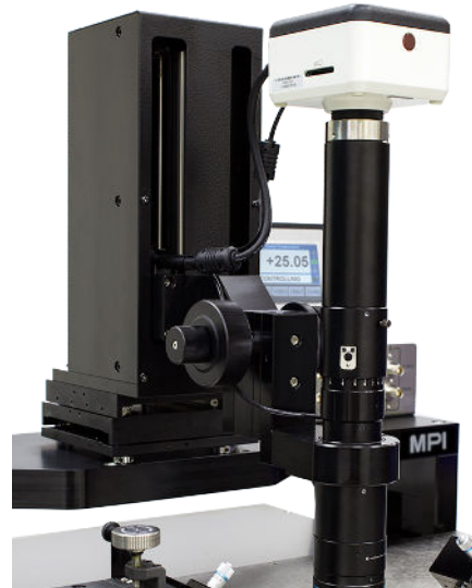
Fig. 9: MegaZoom™ MZ12 microscope with HDMI camera
