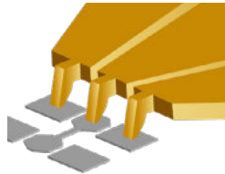
Fig. 14: TITAN™ Probe tip design
