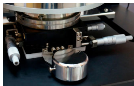
Fig. 7: Air-bearing stage with a single-handed puck control
