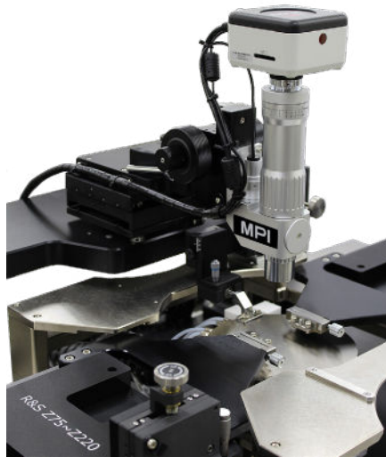
Fig. 8: SuperZoom™ SZ10 microscope with HDMI camera
