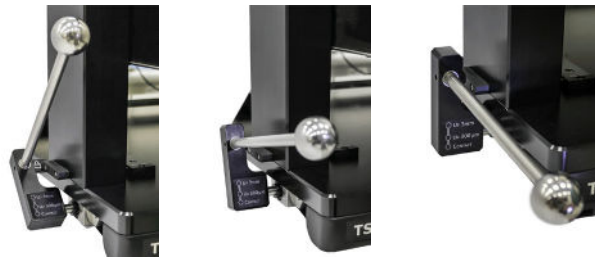
Fig. 12: The platen lift mechanism in three discrete positions: wafer loading (left), separation (middle), and contact (right)
