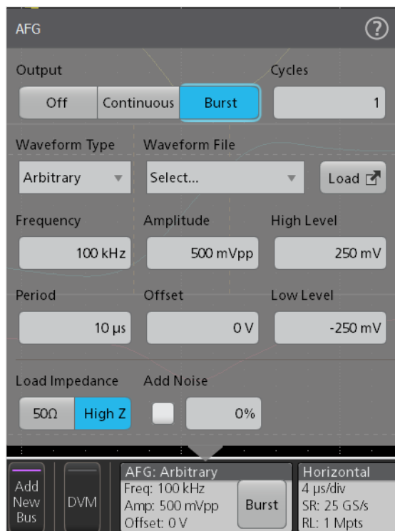
Figure 6: AFG Setup Dialog. For DPT, an arbitrary waveform is used to provide the gate drive signal.
